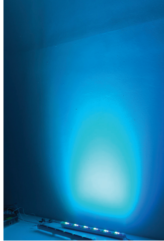
Effect of 20x40deg beam type 20cm away from the wall
