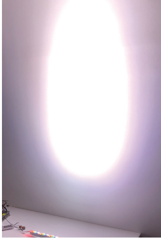
Effect of 16deg beam type 20cm away from the wall
